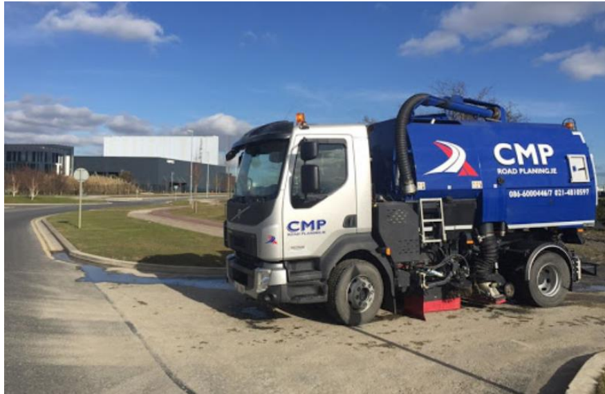
Figure 5.1 Typical road sweeper (Source: CMP Road Planning)
